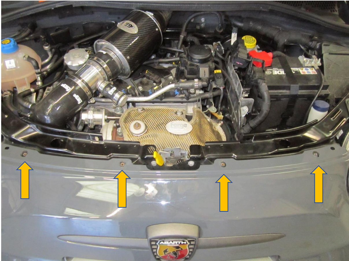
8. Your new Forge Motorsport oil cooler fits in the OEMs intercooler position as pictured below.
